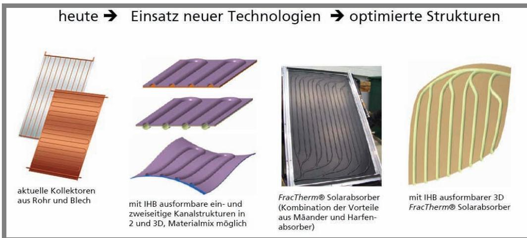
*Optimized structures with forming process by the use of over pressure;*
